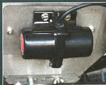
Optional vibrator helps keep material moving.
