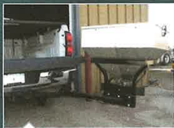
Optional swing-away hitch provides convenient access to the truck bed & tailgate. (Shown on Model SS1000)
